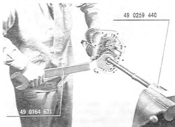
Fig. 7-11 Loosening of lock nut
