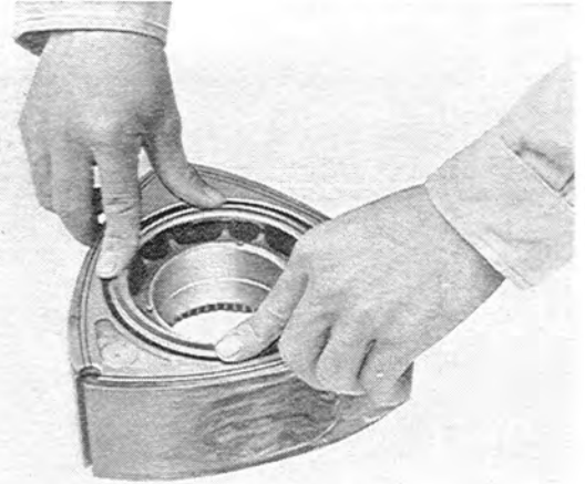
Fig. 1-75 Installing oil seal
