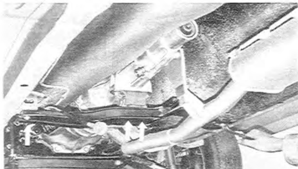
Fig. 7-4 Removing of cross member
