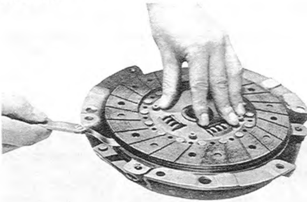
Fig. 6-4 Checking of clutch disk
