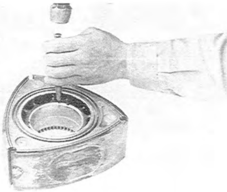
Fig. 1-55 Staking locking screws
