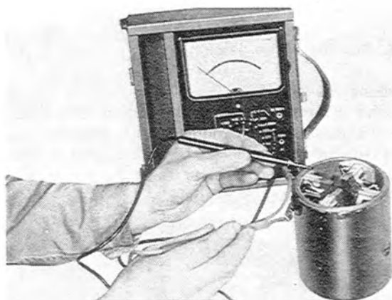
Fig. 5-27 Checking of field coil
