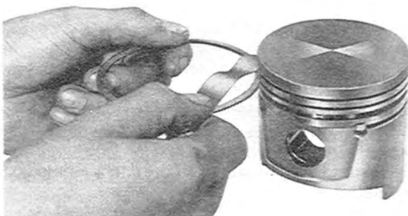
Fig. 1-27 Piston ring groove inspection
