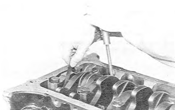
Fig. 1-37 Checking of end play
