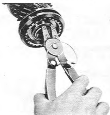
Fig. 7A-13 Installing of snap ring
