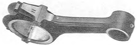
Fig. 1-33 Mark of connecting rod weight
