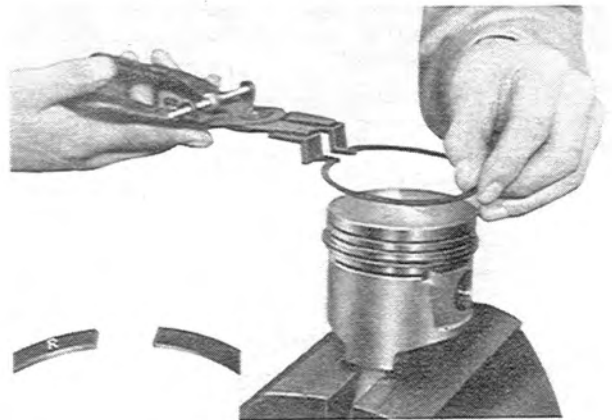
Fig 1-44 Installing of piston ring
