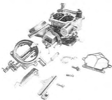
Fig. 4-2 Removing of air horn
