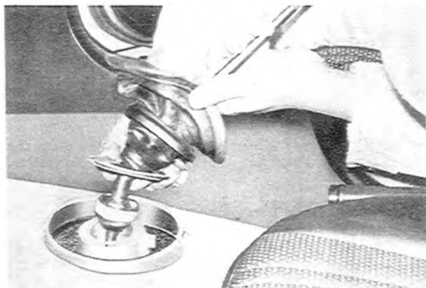
Fig. 7-3 Removing of gearshift lever
