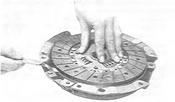
Fig. 6-4 Checking clutch disk
