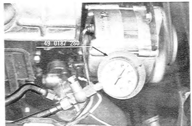
Fig. 2-3 Checking of oil pressure.
