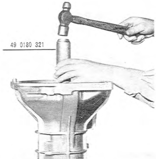
Fig. 7A-20 Installing of bearings
