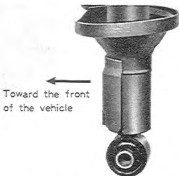
Fig. 13-30 Lower of rear shock absorber
