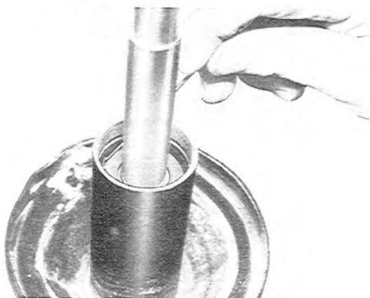
Fig. 13-9 Removing of "O" ring
