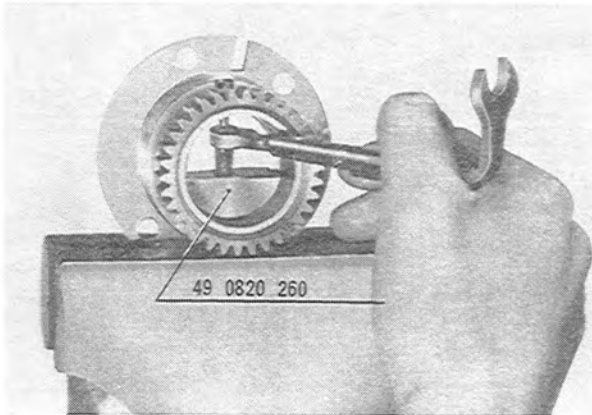
Fig. 1-33 Removing lock pin
