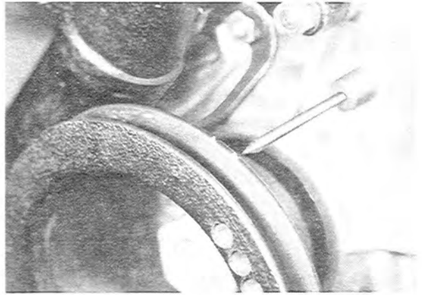
Fig. 1-78 Aligning of crankshaft pulley
