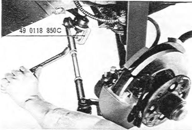
Fig. 10-3 Disconnecting of center link
