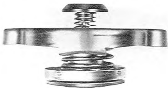
Fig. 3-2 Expansion tank pressure cap
