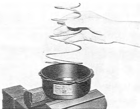
Fig. 11-9 Removing of return spring
