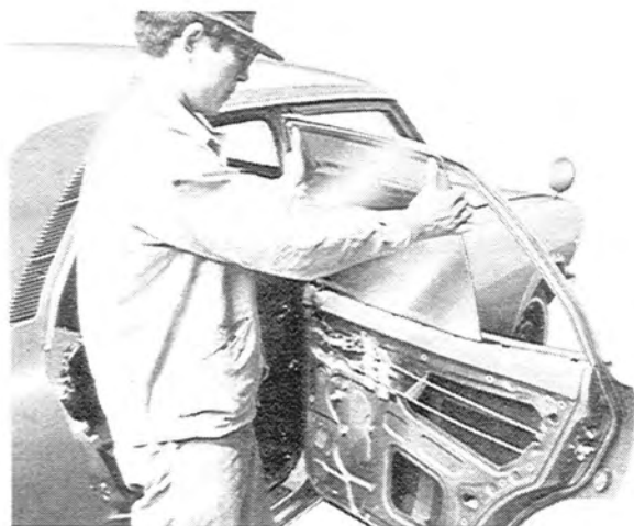
Fig. 14-26 Removing of glass
