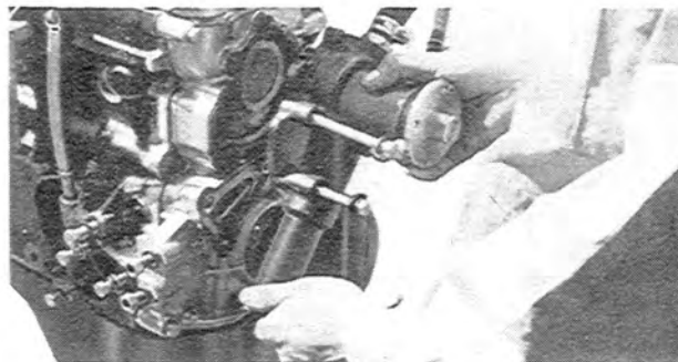
Fig. 1-75 Installing of water pump
