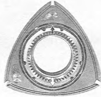
Fig. 1-74 Position of spring gap
