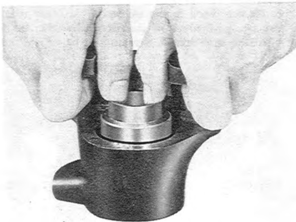
Fig. 11-22 Installing of piston
