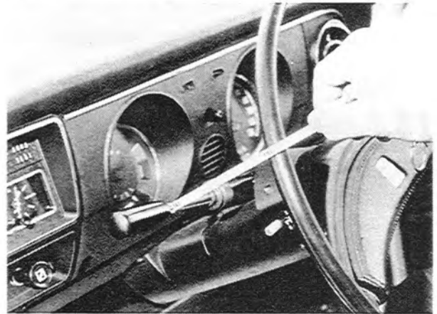
Fig. 7A-24 Change lever adjustment
