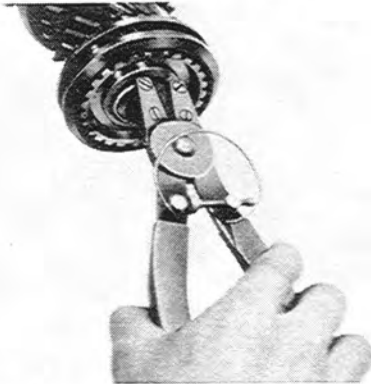
Fig. 7-20 Installing of snap ring
